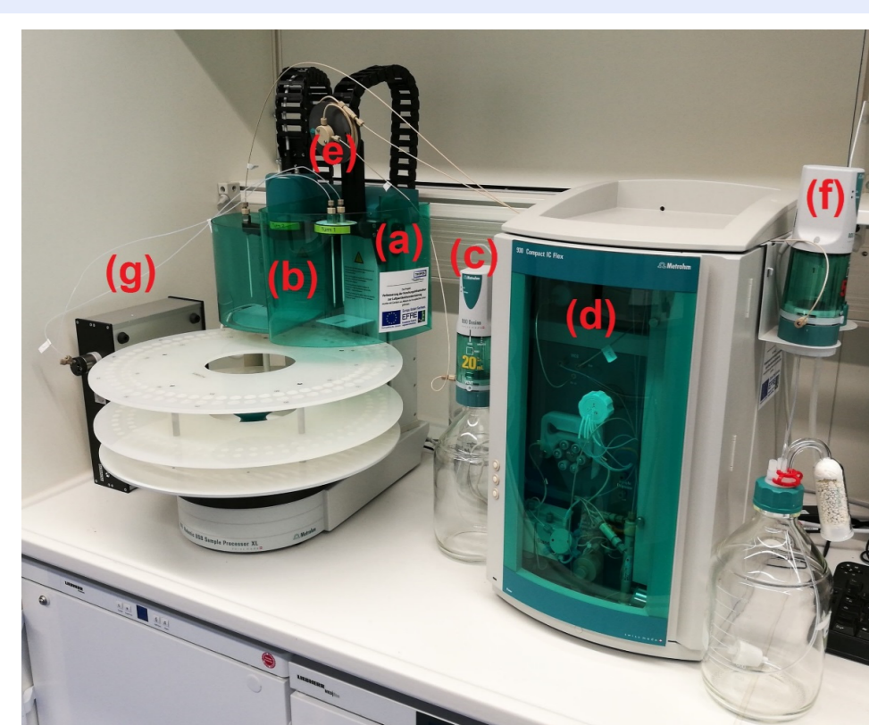
Fig. 1: Setup of the Compact IC system with (a) the first working and (b) the second working station of the autosampler with 120 slots for 12.5 mL vials arranged in two circles. (c) the 800 Dosino for the sample transportation between autosampler and (d) the Compact IC via a 10 mL sample loop (e). A further 800 Dosino (f) for the gradient system. The sample flow between MARGA and Compact IC was controlled by an external six-way valve (g).
