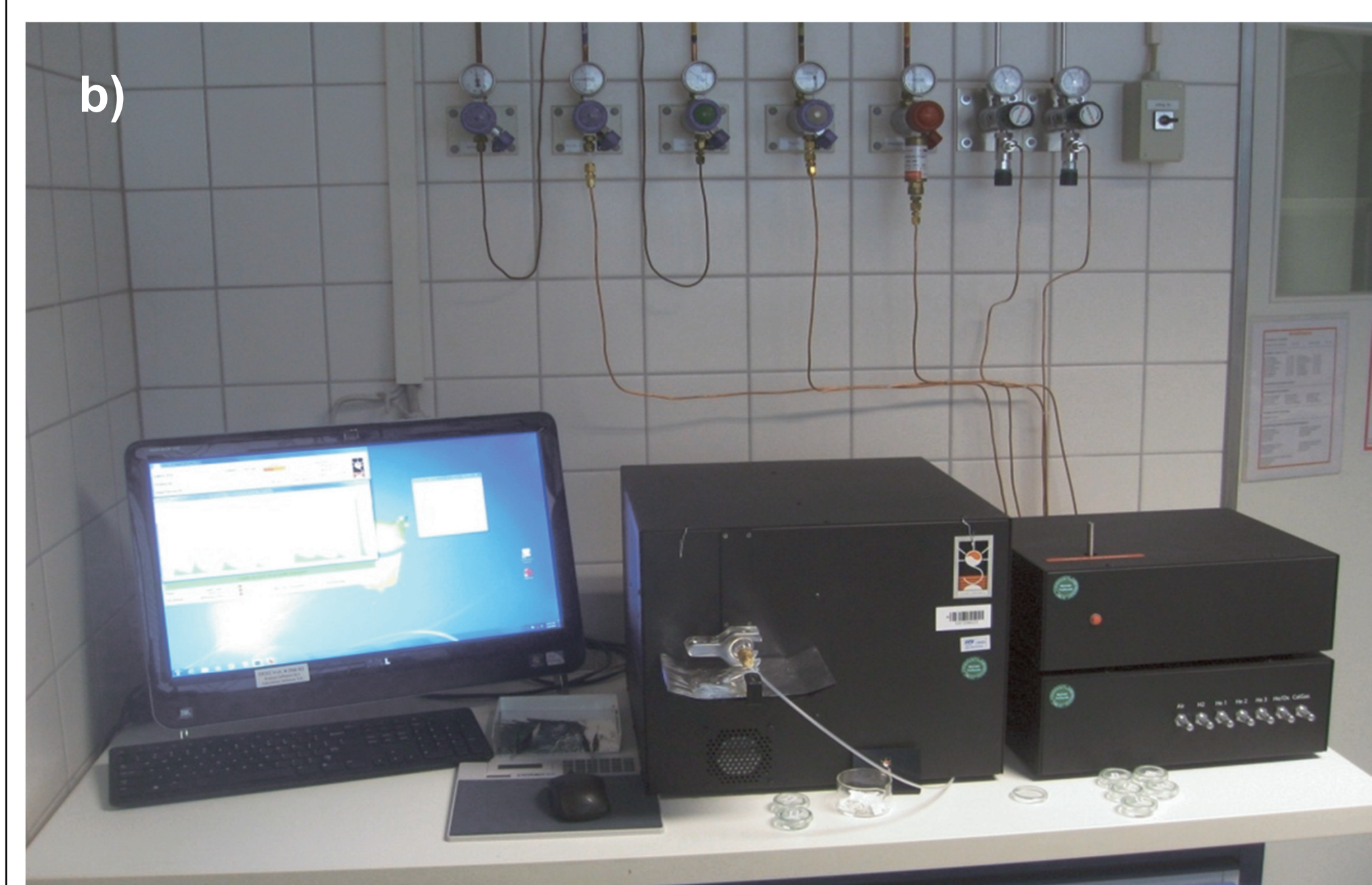
Figure 1: a) OCEC analyzer C/Smax with quartz oven, thermographic method b) OCEC analyzer by Sunset Laboratory Inc., thermo-optical method
