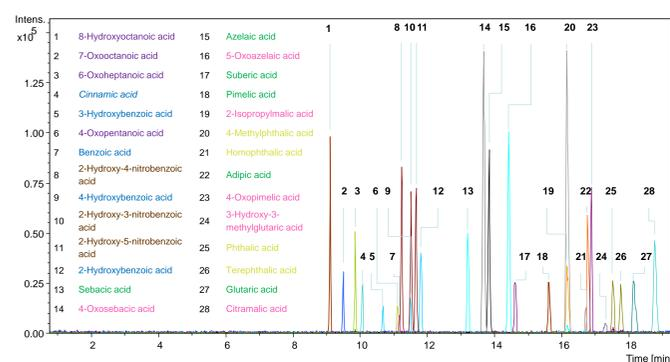
Fig. 2: Example of an electropherogram of a standard solution containing target species.
