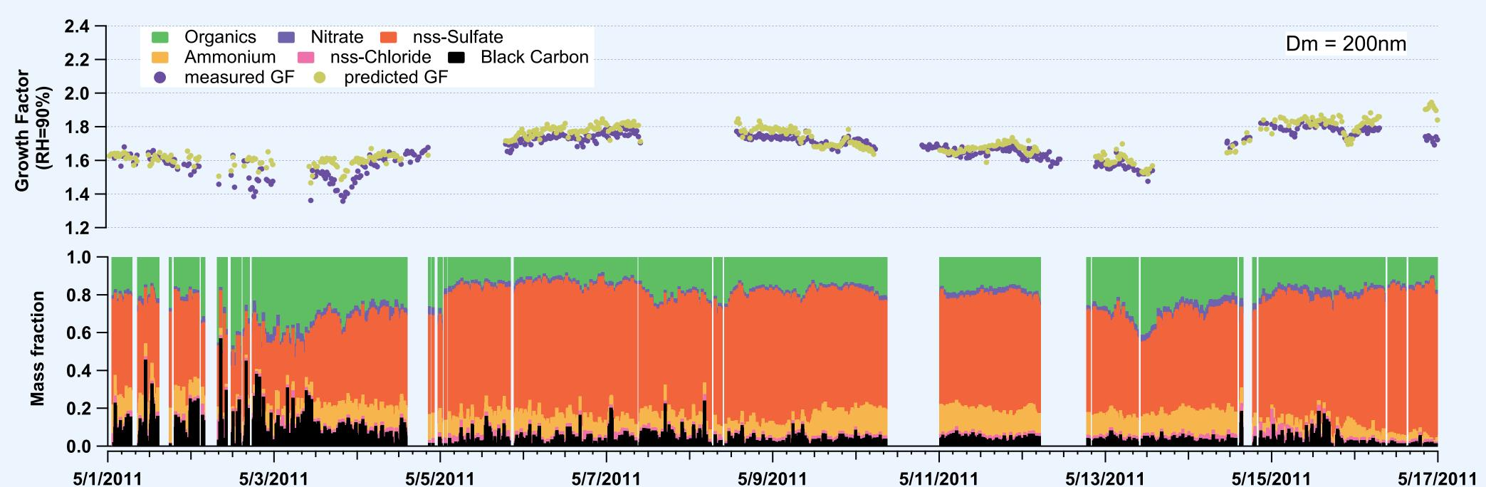
The predicted hygroscopic growth factor (HGF) based on AMS chemical composition could generally fit well with measured GF on 200 nm. But GF was overestimated when nss-sulfate took big portion.
