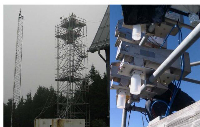
Fig. 1. Cloud water measurement tower during HCCT 2010 with collectors mounted at the sides to SW on top of the tower. Series of backward trajectories during full cloud event FCE 13.3.
