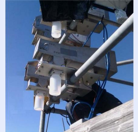
Fig. 1. Stainless steel Caltech Active Strand cloud water collectors mounted parallel to each other on the tower platform.
