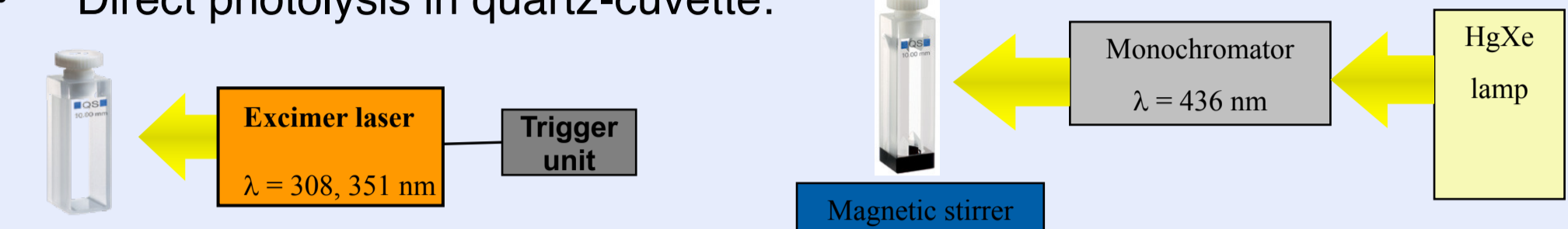
Fig. 2: Experimental setup for complex photolysis with excimer laser (20ns pulse) or HgXe-lamp (continuous irradiation).
