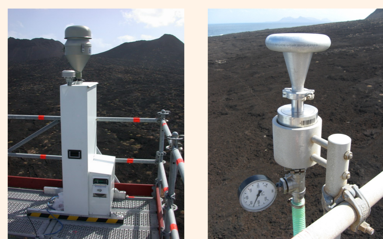
Fig. 2: DIGITEL high volume sampler (left) with PM 10 -inlet, 500 l min -1 , 150 mm quartz fibre filters (Munktell MK 360); BERNER 5-stages impactor (right), 75 l min -1 , collecting on aluminium and Nuclepore ® foil, stages lower cut-offs: 0.05 - 0.14 - 0.42 - 1.2 - 3.5 µm
