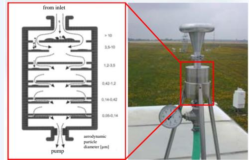
Fig. 1: Five-stage low-pressure cascade impactor (BERNER type), flow rate  $4.5 \text{ m}^3/\text{h}$  at Melpitz site
