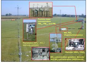
Figure 1: View of the anchor station Melpitz (12°56' E, 51°32' N, 86 m above see level). Measurements for N-containing chemical species are highlighted.
